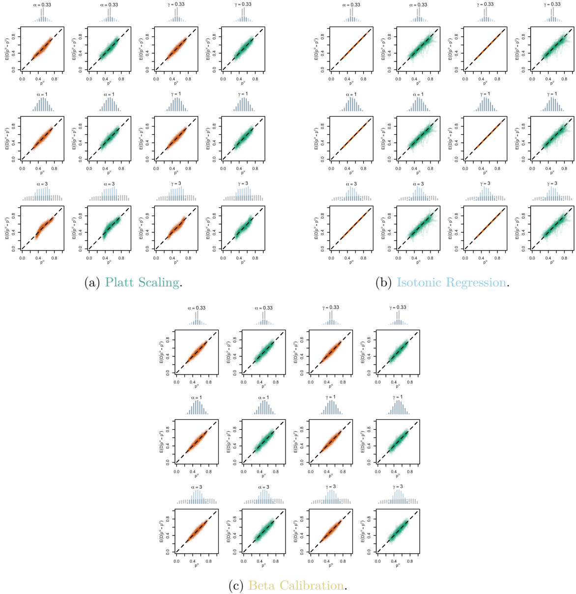
Figure 12: Calibration Curves Calculated with Scores Recalibrated Using Platt Scaling (Panel a), Isotonic Regression (Panel b), or Beta Calibration (Panel c) . The curves are obtained with quantile binning , for the calibration set (orange) and for the test set (green) for varying values of \alpha and \gamma . The curves of the 200 replications of the simulations are superimposed. The histogram on top of each graph show the distribution of the uncalibrated scores (gray) , and that of the calibrated scores (blue) .
